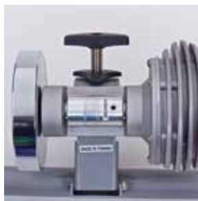
TENSION ADJUSTMENT – No-Slip tension adjuster locks roller in place.
